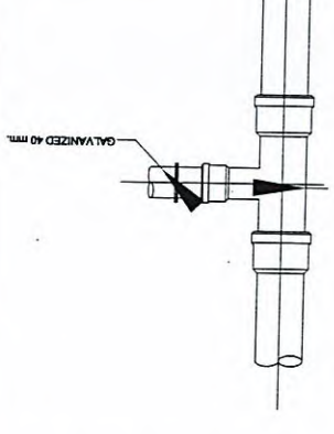
TYPICAL CLEAN OUT FOR MAIN SANITARY STACK TYPE 3
